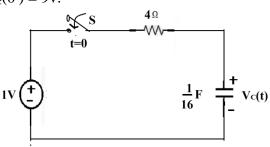
2. a) Derive the Transient Response of series RC-circuit with D.C excitation. [5M]
