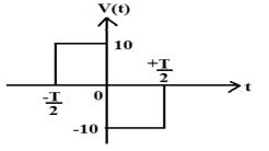
6. a) Find the Trigonometric Fourier series for the waveform shown in figure and sketch the spectrum.
